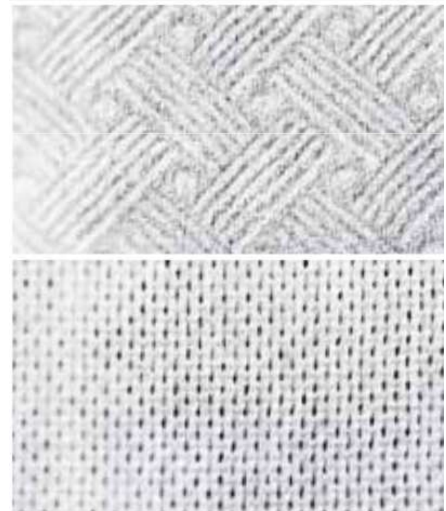
Structured (top) and perforated web (below)
