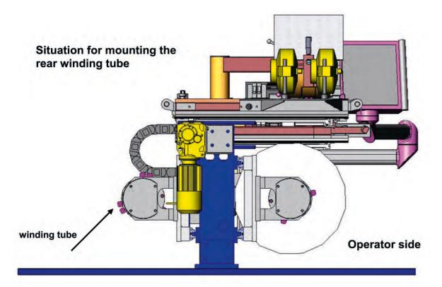
After retracting the table plate, the spiral screen to be filled which is wound up on a winding tube is inserted on the operator side.
