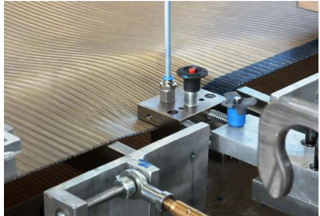
Image 6 Ideal height setting for glue nozzle
