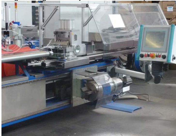
Sliding bearing unit with jaw chuck on the operator side
