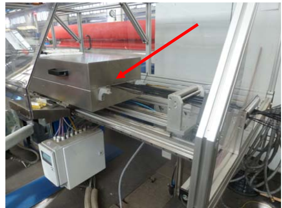
Filler wire fixing box (view from operator side)
