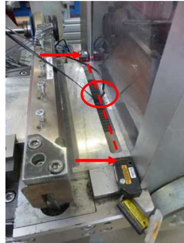
Filler wire monitoring with photocell
