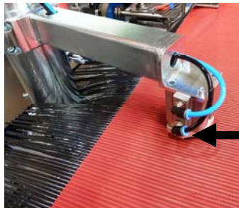
Precursor (fixed with sleeve bracket)
