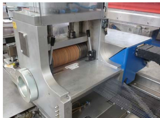
Drive unit with open protective panel (pintle wire side)
