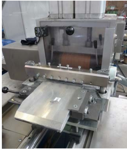
Drive unit with cutting unit and template (sleeve side)
