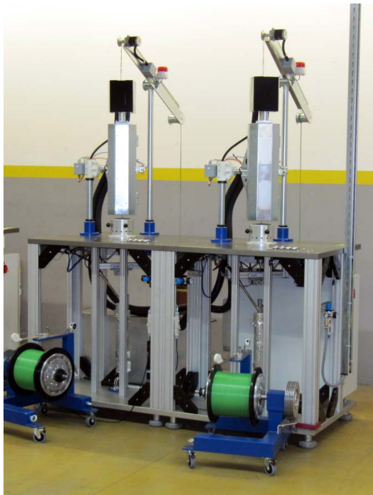
High performance spiral machine with independently operating right and left spindles
