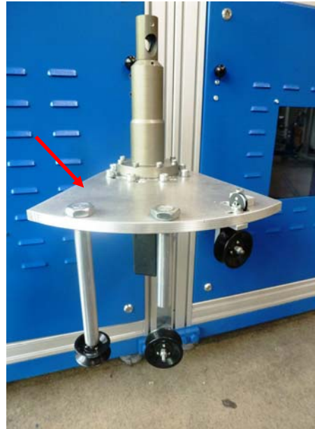
Winding plate (for round monofilament)
